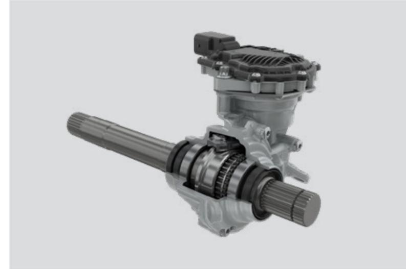
electromechanical device that disconnects the e-motor from the driveshaft in EVs when propulsion power is not needed, reducing energy consumption, and increasing efficiency. It contributes to increased electric driving range of up to nine percent, a significant benefit for all EVs. This is achieved by reducing drag torque losses of the e-motor and gearbox
